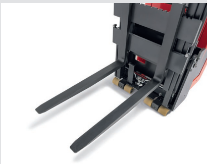
Fitted with ISO standard forks, the trucks can handle all types of pallets
